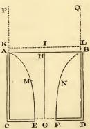
ABNFEM, passing through the hole EF, and filling up the same exactly. Let the uniform velocity of the descending ice and of the contiguous water in the circle AB be that which the water would acquire by falling through the space IH; and let IH and HG lie in the same right line; and through
