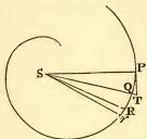
Let that spiral be PQR. From the velocity, with which the body goes over the very small are PQ, the time will be given; and from the altitude TQ, which is as the centripetal force, and the square of the time, that force will be given. Then from the difference RSr of the areas PSQ and GSR described in equal particles of time, the retardation of the body will be given; and from the retardation will be found the resisting force
