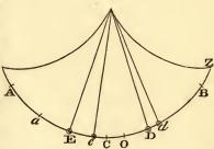
half of that difference Aa. Therefore the force with which the oscillating body is urged at the beginning or the highest point of the cycloid, that is, the force of gravity, will be to the resistance as the arc of the cycloid, between that highest point and lowest point C, is to the arc CO; that is (doubling those arcs), as the whole cycloidal arc, or twice the length of the pendulum, to the arc Aa. Q.E.D.
