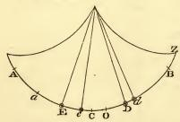
Let AB be an arc of a cycloid, which a body D, by vibrating in a non-resisting medium, shall describe in any z time. Bisect that arc in C, so that C may be the lowest point thereof; and the accelerative force with which the body is urged in any place D, or d or E, will be as the length of the arc CD, or Cd, or CE. Let that force be ex-
