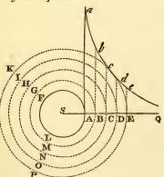
CASE 1. Let AFL be a sphere turning uniformly about the axis S, and let the concentric circles BGM, CHN, DIO, EKP, &c., divide the fluid into innumerable concentric orbs of the same thickness. Suppose those orbs to be solid; and, because the fluid is homogeneous, the impressions which the contiguous orbs make one upon another will be (by the supposition) as their translations from one another, and the contiguous superficies upon which the
