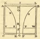
CASE 6. If the lower part of the vessel ABDC B be immersed into stagnant water, and the height of the stagnant water above the bottom of the vessel be GR, the velocity with which the water that is in the vessel will run out at the hole EF into the stagnant water will be the same which the water would acquire by falling from the height IR; for the weight of all the water in the vessel that is below the superficies of the stagnant water
