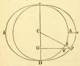
allel lines, they will generate the parallel heights Ff, Aa, in the same ratio; and therefore the figure of the water Dfaeb will be a spheroid made by the revolution of an ellipsis about its longer axis ab. And the perpendicular height fh will be to the oblique height Ff as fG to /C, or as FG to AC: and therefore the height fh is to the height Aa in the duplicate
