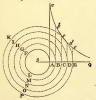
Let AFL be a cylinder turning uniformly about the axis S, and let the concentric circles BGM, CHN, DIO, EKP, &c., divide the fluid into innumerable concentric cylindric solid orbs of the same thickness. Then, because the fluid is homogeneous, the impressions which the contiguous orbs make upon each other mutually will be (by the Hypothesis) as their translations from each other, and as the contiguous superficies upon which the impressions
