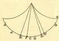
For let equal pendulums in a resisting medium describe the unequal arcs A, B; and the resistance of the body in the arc A will be to the resistance of the body in the correspondent part of the arc B in the duplicate ratio of the velocities, that is, as, AA to BB nearly. If the resistance in the arc B were to the resistance in the arc
