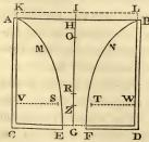
Therefore in what follows let the diameter of the stream be represented by that lesser hole which we called EF. And imagine another plane VW above the hole EF, and parallel to the plane thereof, to be placed at a distance equal to the diameter of the same hole, and to be pierced through with a greater hole ST, of such a magnitude that a stream which will exactly fill the lower hole EF may pass through it; the diameter of which hole
