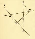
From the given point P suppose any right line PD to be drawn to either of the right lines given, as AB; and produce the same towards AC, the other given right line, as far as E, so as PE may be to PD in the given proportion. Let EC be parallel to AD. Draw CPB, and PC will be to PB as PE to PD. Q.E.F.
